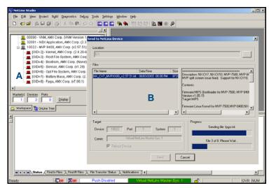
FIG. 38 Using USB for a Virtual Master transfer
